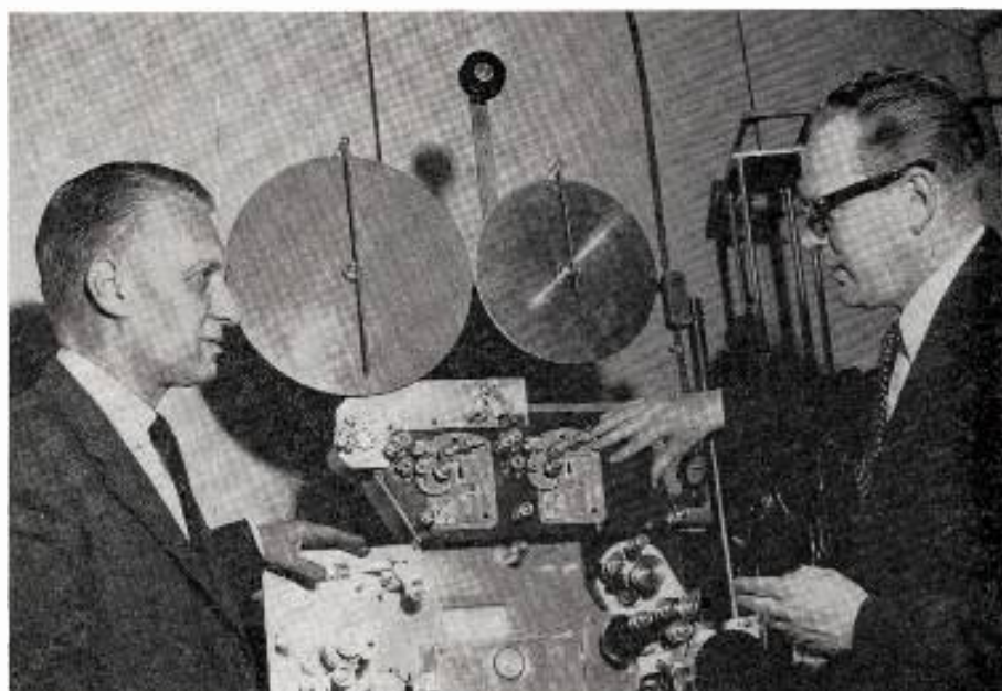
HOWARD L. KANY (left), manager of newsfilm, CBS News, learns from inventor R. C. Rheineck , chief engineer, CBS News, how this custom-built prototype of a magnetic stripe film printer operates at Du Art Film Labs., New York. Mr. Rheineck's right hand is pointing to assembly which makes magnetic print directly from magnetic original (both film picture and magnetic sound stripe). Assembly below this makes regular optical sound-and-picture print from magnetic original.
